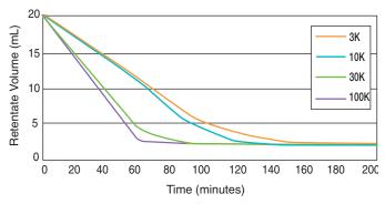
Protein solutions were processed in each of the Macrosep Advance devices. Average time (minutes) is plotted against mL of remaining product to be filtered using a swinging bucket rotor at 5,000 g. Solutions are 3K: Protamine Sulfate, 0.1% in 1X PBS; 10K: Cytochrome C, 0.025% in 1X PBS; 30K: IgG, 0.1% in 1X PBS; and 100K: Apoferitin, 0.1% in 1X PBS.
