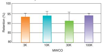
Protein solutions were processed in each of the Microsep Advance devices. Average percent retention using 34° fixed angle rotor at 5,000 g is displayed for each MWCO. Solutions were 3K: Cytochrome C, 250 µg/mL; 10K: BSA, 1 mg/mL; 30K: IgG, 1 mg/mL; and 100K: thyroglobulin, 1 mg/mL.
