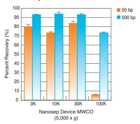
A 500  $\mu$ L sample of a 100  $\mu$ g/mL DNA fragment solution containing 50 and 500 bp double-stranded DNA fragments was centrifuged at 5,000 x g in Nanosep devices to a final volume of 50  $\mu$ L. Recovered samples were quantified using absorbance at 260 nm. The 100K device was able to differentiate between the sizes of the DNA fragments.
