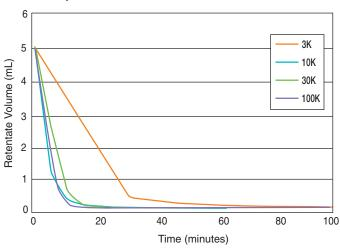
Protein solutions were processed in each of the Microsep Advance devices. Average time (minutes) is plotted against mL of remaining product to be filtered using a 34° fixed angle rotor at 5,000 g. Solutions are 3K: Cytochrome C, 250 µg/mL; 10K: BSA, 1 mg/mL; 30K: IgG, 1 mg/mL; and 100K: Thyroglobulin, 1 mg/mL.
