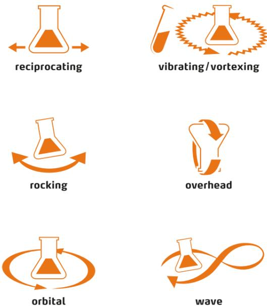
Six different shaking motions – from one- to three-dimensional. Individual movements in addition vary in their motion amplitudes and tilt angles.
