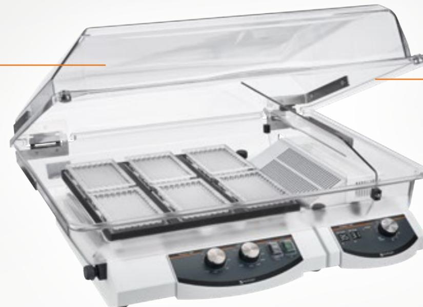
Full visual reaction control through the transparent PETG incubation hood, which does not allow condensation to form
