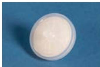
Designed for filtration and purification in a sterile environment. Fisherbrand™ Sterile PES Syringe Filter features a PES membrane in a polypropylene housing for purification of tissue culture solutions from a standard syringe. 33mm diameter membranes available with 0.2 or 0.45µm pore sizes.
