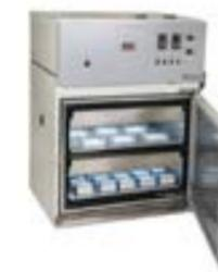
Temperature Range: 0°C to 60°C with light, 10°C to 50 C without light; Relative Humidity (RH): <95% with Light Off at 37°C; <75% with Light On at 37°C; Light: Optional Fluorescent Light Module. Thermo Scientific™ Vertical Light Chambers address a variety of applications that require sample exposure with light, along with temperature control
