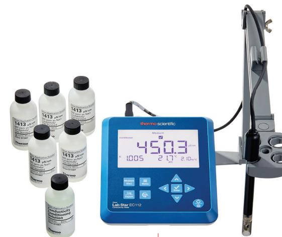
For a wide variety of conductivity samples in the 1  $\mu\text{S}/\text{cm}$  to 20  $\text{mS}/\text{cm}$  range.
