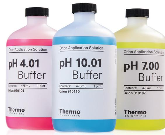
Orion pH buffers and ORP standards are traceable to NIST standard reference materials and are labeled with a lot code and expiration date.
