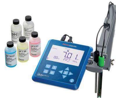
**Select the low-maintenance bio kit (Cat. No. LSTAR1117)** for samples containing TRIS buffers, proteins, sulfides, halides or other components that can interfere with silver chloride. This gel-filled pH electrode is low-maintenance and easy to operate.
