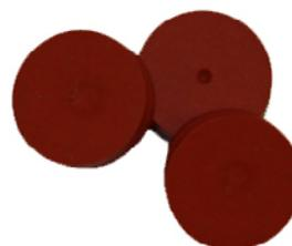
The purpose of a septa in a GC system is to isolate the sample flow path from the outside world. The septa provides a barrier that is readily penetrated by the injector needle whilst maintaining internal pressure without causing system contamination. An ideal septa has low bleed and a long lifetime.
