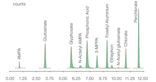
Figure 3. The typical chromatogram obtained after a 15 μL injection of 100 ppb standard solution on the Acclaim Trinity P1 column
