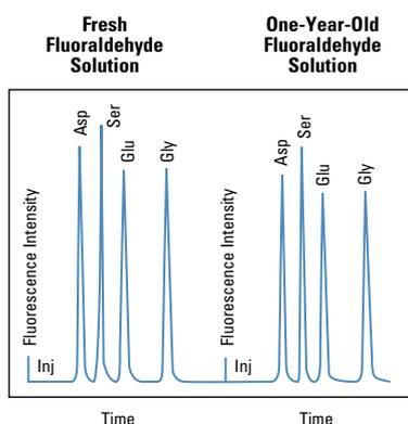
**Figure 2. Outstanding shelf life.** Comparison of fluorescence response of selected amino acids after reaction with recently prepared and one-year-old Thermo Scientific Pierce Fluoraldehyde Reagent Solutions.
