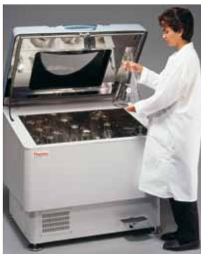
to 2 inches (5.1 cm). The size of the orbit will affect how the bacterial cells circulate and how the growth medium is aerated. It turns out that shaker orbit diameter has a linear relationship to the Oxygen Transfer Rate (OTR)<sup>4</sup>, which is the rate at which oxygen gas is transferred from the air to the liquid. Thus, if the orbital shaker diameter doubles, so does the OTR.
