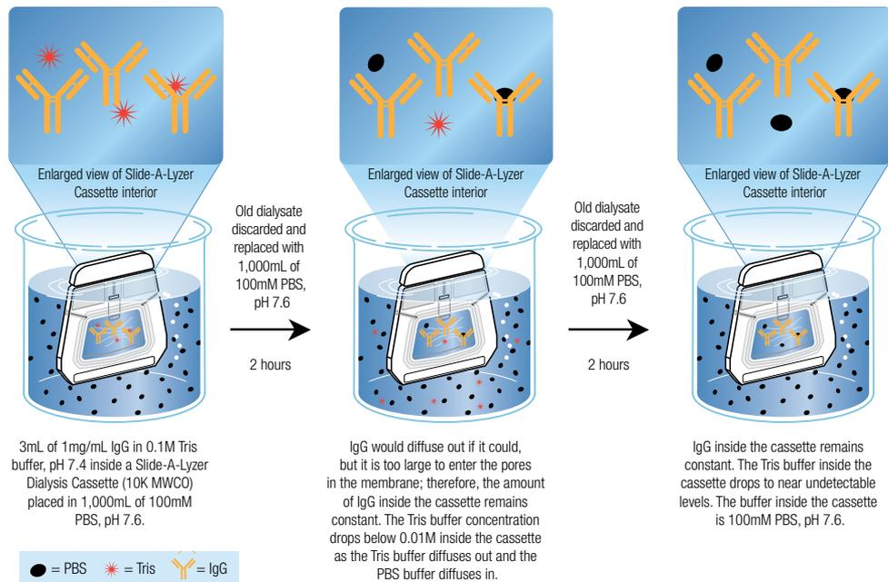
Figure 2. How the Thermo Scientific Slide-A-Lyzer Cassette works.
