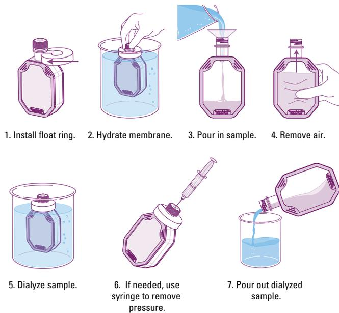
**Figure 1. Easy sample loading and recovery.** Attach supplied float-ring and hydrate membrane for 2 minutes. Pour sample into device. Remove air and cap. Dialyze for 8 hours to overnight (replace buffer after 2 and 5 hours). Pour out sample to recover.
