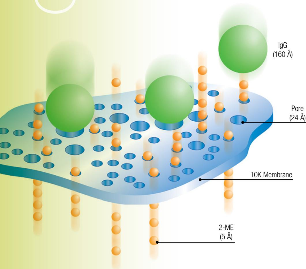
**Figure 1. How dialysis membranes work.** A dialysis membrane is a semi-permeable film (usually a sheet of regenerated cellulose) containing various sized pores. Molecules larger than the pores cannot pass through the membrane, but small molecules can do so freely. In this manner, dialysis may be used to perform purification or buffer exchange for samples containing macromolecules.
