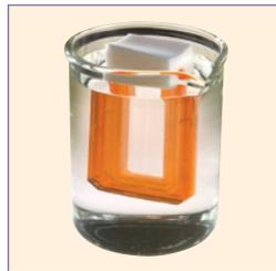
2. Attach a float buoy and dialyze. (Buoys also serve as convenient bench-top stands for the cassettes.)
