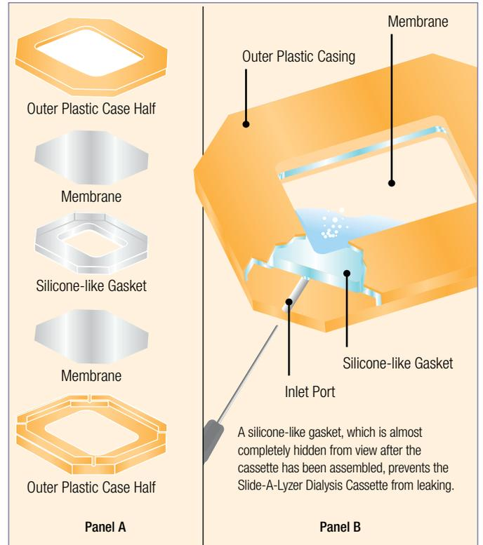
Figure 2. Thermo Scientific Slide-A-Lyzer Cassette design. The Slide-A-Lyzer Dialysis Cassette (exploded view) looks like a sandwich (Panel A). When all of the pieces are compressed together (Panel B), the outer plastic case halves are welded together sonically, hermetically sealing an inner chamber that can be accessed only via a syringe needle inserted through the inlet port. Because the inert gasket is 10mm wide, the needle path is sealed completely and tightly when the syringe is withdrawn.
