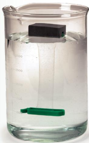
SnakeSkin Dialysis Tubing is an easy- and ready-to-use form of traditional dialysis membrane tubing that allows desalting and buffer exchange for 10 to 100mL samples, and it does not require presoaking or boiling prior to use. To use, simply pull out and cut off the required length of tubing, fold over one end of tubing and close with a dialysis clip, add sample at the open end, and use a second clip to close the remaining end.
