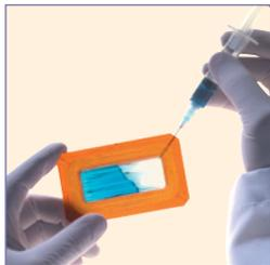
1. Insert syringe needle through the gasket via one of the corner ports. Inject the sample, withdraw the excess air and remove the syringe.
