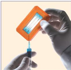
3. Insert empty syringe needle at a second corner port. Inject air to expand the cassette chamber, then withdraw the dialyzed sample.
