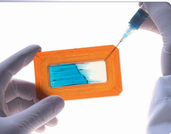
The Slide-A-Lyzer Dialysis Cassettes are available in five membrane MWCOs (2K, 3.5K, 7K, 10K and 20K) and in four different sizes for dialyzing sample volumes between 0.1 and 30mL. Slide-A-Lyzer Cassettes can be used for a wide range of applications, including low-molecular weight contaminant removal, buffer exchange, desalting and sample concentration.
