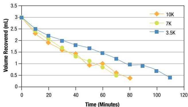
**Figure 1. Rapid sample concentration.** Slide-A-Lyzer Concentrating Solution quickly reduces a starting volume of 3mL of sample inside the Slide-A-Lyzer Dialysis Cassette to 0.5mL in about 50 minutes.
