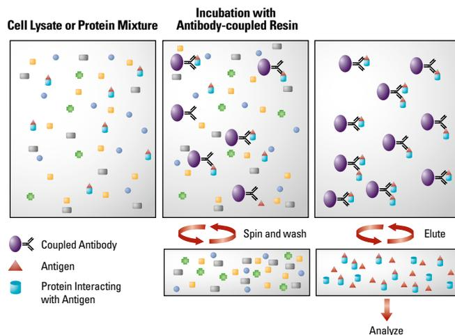
Figure 2. Summary of a traditional co-immunoprecipitation procedure.
