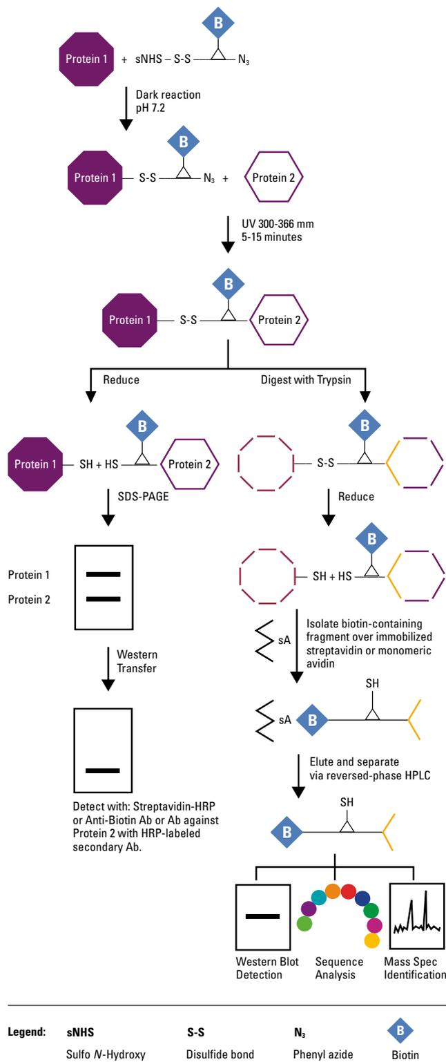
Figure 10. Applications of Thermo Scientific Pierce Sulfo-SBED in protein interaction studies.
