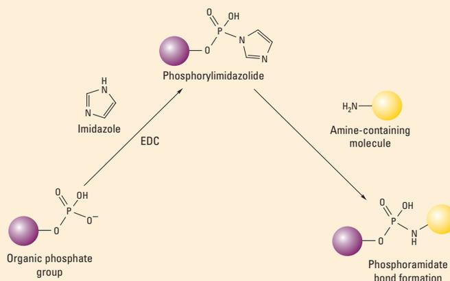
**Figure 13.** Reaction scheme showing typical route to conjugating an amine-containing biomolecule to a 5' terminal phosphate group.
