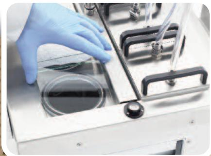
**Sealed bath surface** prevents the bath fluid from condensing on the glass plate
