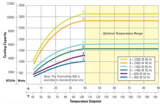
Cooling capacity based on chillers with P2 pumps set at 10 gpm. Other pumps and flow rates will affect cooling capacity performance.
