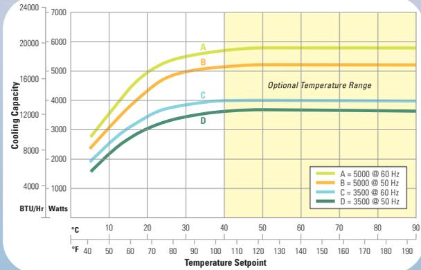
Cooling capacity based on chillers with P2 pumps with no backpressure. Other pumps will affect cooling capacity performance.
