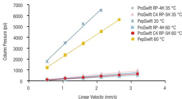
Figure 1: Column backpressure as a function of eluent flow rate at 35 °C and 60 °C for a ProSwift RP-4H, a ProSwift C4 RP-5H column, and a PepSwift column. All column formats are 100  $\mu\text{m}$   $\times$  25 cm, eluent: 90.5/9.5 water/acetonitrile + 0.1% trifluoroacetic acid
