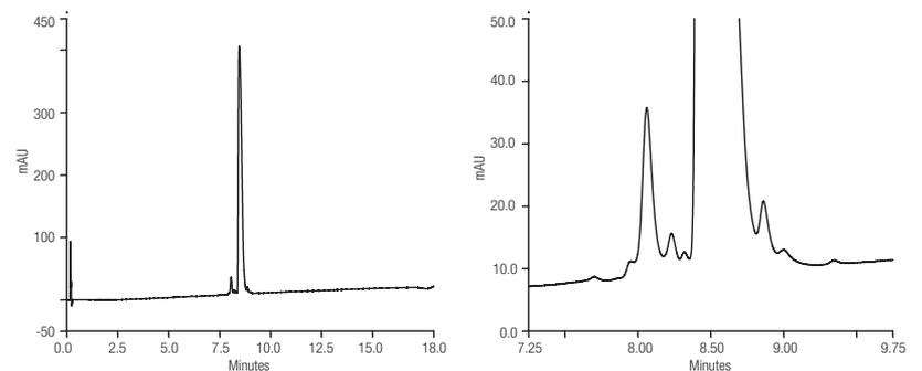
Figure 8: Separation of mAb variants using a 500  $\mu\text{m} \times 10\text{ cm}$  ProSwift C4 RP-5H column. The separation was performed at a temperature of 85  $^{\circ}\text{C}$  and a flow rate of 150  $\mu\text{L}/\text{min}$  using a gradient from 12–55% B over 15 minutes with 97.5/2.5 (v/v) water/acetonitrile + 0.1% trifluoroacetic acid for eluent A and 10/90 water/acetonitrile + 0.08% trifluoroacetic acid for eluent B.
