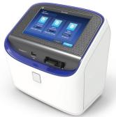
variation associated with manual focusing mechanisms. The Countess II FL Automated Cell Counter offers bright-field and two optional, user-interchangeable fluorescent channels. The fluorescent colours collected are determined by the insertion of individual light cubes.
