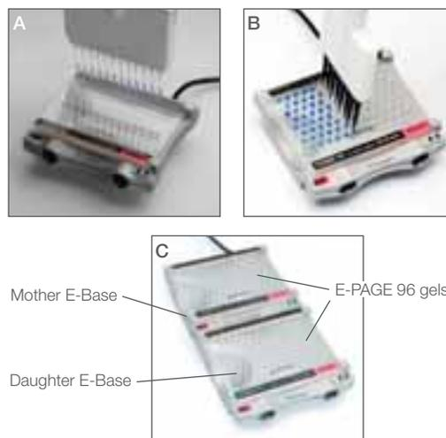
**Figure 20. Loading and running E-PAGE gels.** (A) Loading E-PAGE 48 gels using a multi-channel pipettor. (B) Loading E-PAGE 96 gels using a multi-channel pipettor. (C) The Mother/Daughter E-Base combination.
