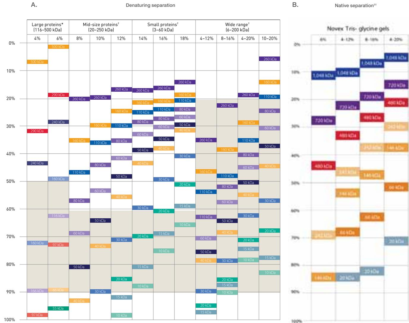
**Figure 11. Migration patterns of protein molecular weight standards in Novex Tris-glycine gels.** For optimal results, protein bands should migrate within the gray shaded areas. **(A)** \*Migration patterns of HiMark™ Unstained Protein Standard. †Migration patterns of Novex Sharp Pre-Stained Protein Standard or Novex Sharp Unstained Protein Standard. **(B)** ††Migration pattern of NativeMARK Unstained Protein Standard.
