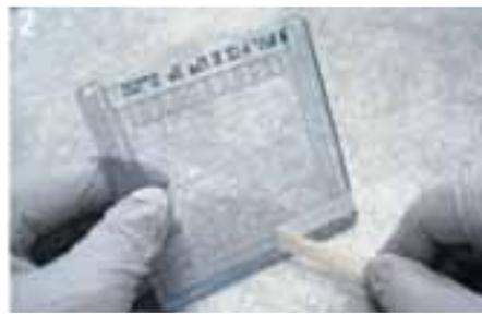
2. Remove the comb, and peel away the tape at the bottom of the gel cassette. Rinse the wells 3 times with 1X buffer.
