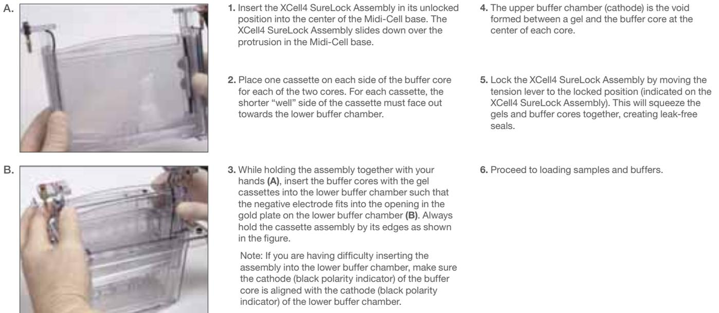
Figure 28. How to use the XCell4 SureLock Midi-Cell with 4 gels.
