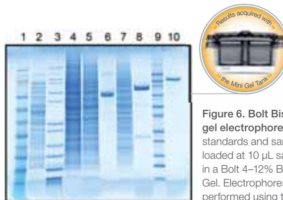
**Figure 6.** Bolt Bis-Tris Plus gel electrophoresis. Protein standards and samples were loaded at 10  $\mu$ L sample volumes in a Bolt 4–12% Bis-Tris Plus Gel. Electrophoresis was performed using the Mini Gel Tank at 200 V (constant). Sharp,
