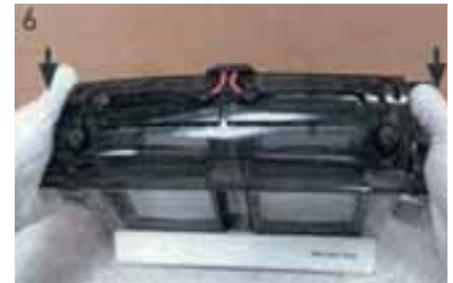
6. Make sure the power supply is off. If only running one gel, remove the cassette clamp from unused chamber. Place the lid on the tank and plug the electrode cords into the power supply. Turn the power supply on to begin electrophoresis.
