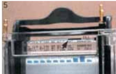
5. Hold the cassette and release the cassette clamp. Gently lower the cassette so that it rests on the bottom of the chamber, and close the cassette clamp. Add 1X buffer to the level of the fill line.
