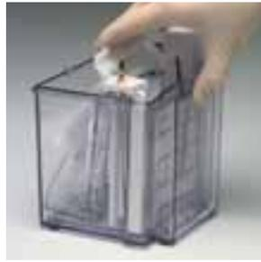
2. Lock the gel tension wedge in place, load samples, and fill the buffer chambers with the appropriate running buffers.
