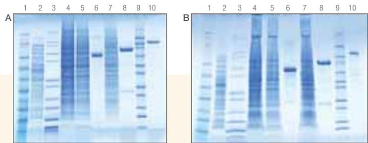
**Figure 4.** Protein separation using (A) a Bolt Bis-Tris Plus gel and (B) another manufacturer's traditional Tris-glycine gel.
