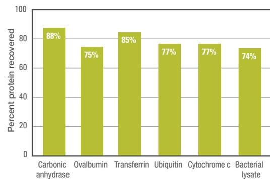
**Figure 23. Consistent protein recovery is achieved using the Pierce SDS-PAGE Sample Prep Kit.** Pure proteins (60 µg) of assorted molecular mass
