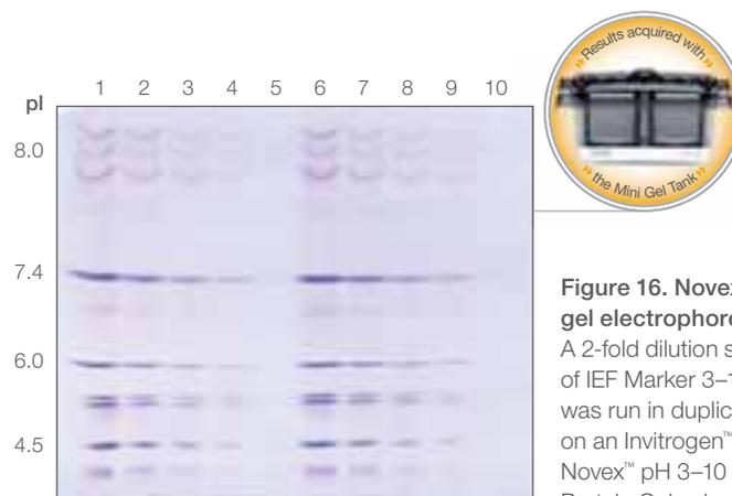
**Figure 16. Novex IEF gel electrophoresis.** A 2-fold dilution series of IEF Marker 3–10 was run in duplicate on an Invitrogen™ Novex™ pH 3–10 IEF Protein Gel using
