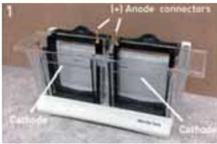
1. Snap the electrophoresis tank into the base, and place the cassette clamp(s) into the chamber(s) with the anode connector(s) (+) aligned to the center. Fill the chamber(s) with 1X buffer to the level of the cathode.
