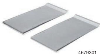
**Heater Covers.** Provide barrier layer between labware and heating coils. Unique design provides additional filtration layer to protect from broken glass. 304 stainless steel. Overall dimensions: 22.5" w x 20.4" d x 2.0" h. Shipping weight 6.0 lbs. (2.7 kg)
