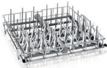
**Upper Spindle Racks.** 304 stainless steel. Includes 36 removable spindles, 36 adjustable height clips, 18 plastic glassware holders, 10 small spindles with clips, 36 spindle plugs, 12 spindle arm plugs and wash arm. Spindles or spindle arms may be removed and plugged to accommodate accessory inserts (sold separately). Spindle dimensions: 4.5" h x 0.25" OD. Overall dimensions: 20.8" w x 21.6" d x 6.9" h. Accommodate glassware up to 8.9" h.
