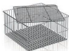
**4573100—Utensil Basket.** For miscellaneous labware such as stoppers, spatulas and other small lightweight items. Includes cover. 304 stainless steel. Overall dimensions: 8.9" w x 8.9" d x 4.0" h. May use up to four per rack at one time. For use in Upper or Lower Standard or Spindle Racks. Shipping weight 3.0 lbs. (1.4 kg)
