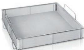
**4573400—Mesh Basket.** Full-sized, open mesh basket can be used for a variety of utensils and loose labware. 304 stainless steel. Overall dimensions: 18.6" w x 19.0" d x 6.7" h. May use one per rack at one time. For use with Upper or Lower Standard Racks. Shipping weight 5.0 lbs. (2.3 kg)
