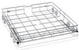
**4669000—Lower Standard Rack.** One is included with every SteamScrubber. May be used in place of Lower Spindle Rack in any FlaskScrubber or FlaskScrubber Vantage. 304 stainless steel. Add accessory inserts to suit your glassware mix (sold separately). Overall dimensions: 21.4" w x 20.9" d x 3.5" h. Shipping weight 12 lbs. (5 kg)
