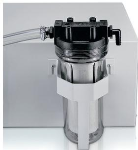
**Chemical Trap.** Traps are connected between the cold trap and the accessory vacuum pump to provide additional protection to the vacuum pump.
