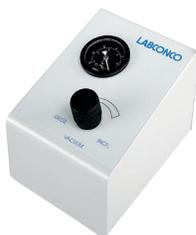
**7991000—Vacuum Controller.** Provides manual control and monitoring of vacuum levels. Analog gauge shows vacuum from 0-30" Hg. At the end of concentration, the control valve may be opened to break the vacuum. **For use with Diaphragm Vacuum Pumps only.** Shipping weight 3.0 lbs. (1.4 kg)
