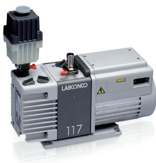
**Rotary Vane Direct Drive Vacuum Pumps.** These pumps are two-stage and oil-sealed with gas ballast control. Isolation valve seals the inlet to prevent oil and air contamination of the system in the event of power failure. Oil mist exhaust filter, vacuum pump oil and inlet adapters suitable for 1/2" OD and 3/4" OD are provided.
