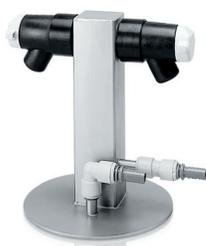
**7397700—Two-Port Manifold.** Has neoprene rubber valves to allow freeze drying of small volume samples in freeze dry flasks, serum bottles or ampules. Connects to CentriVac Cold Trap, Ultra-Low Cold Trap or Mobile System. **Requires use of Rotary Vane Pump.** Not compatible with pre-2005 Cold Traps or Mobile Systems. Shipping weight 1.0 lb. (0.5 kg)
