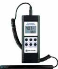
Traceable™ Memory Hygrometer/Thermometer
