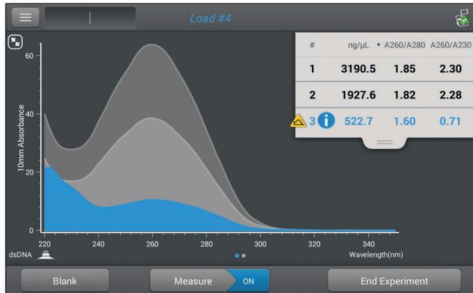
View multiple samples at once on your measurement screen. Here Acclaro has flagged dsDNA sample #3 for the presence of a contaminant.
