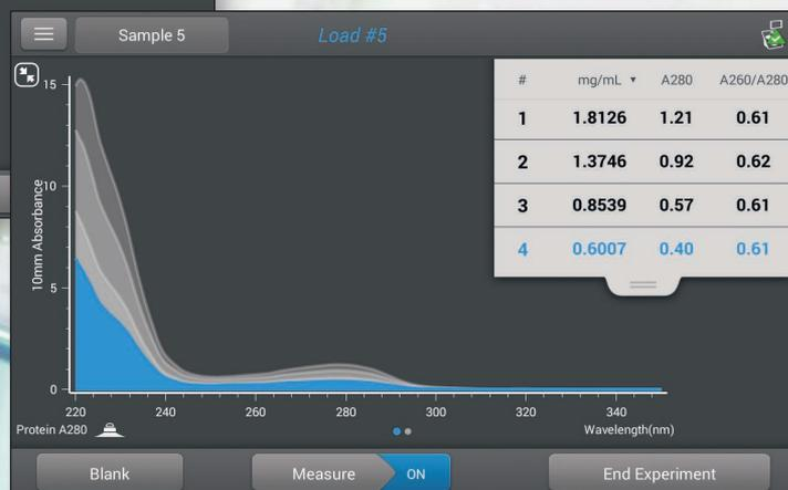
Four different purified protein samples were measured using the Protein A280 application.
