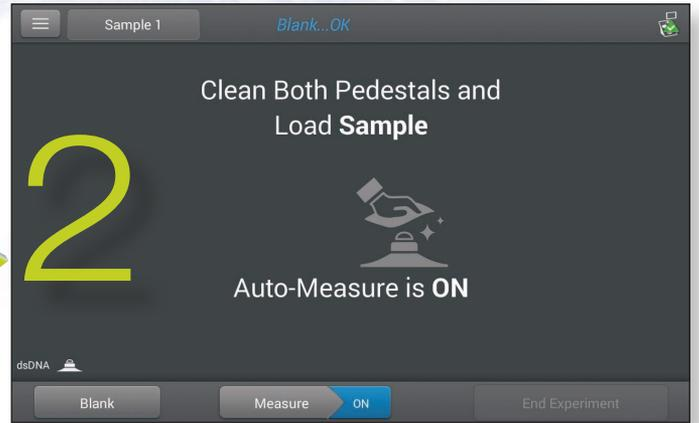
After blanking, load 1–2  $\mu\text{L}$  of your sample and lower the arm. Measurement results with full-spectral data will be displayed in seconds. Swipe left to view expanded data table.
