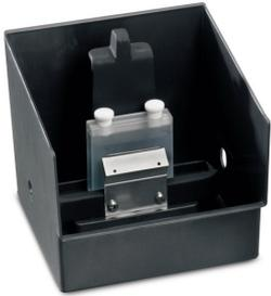
The sample compartment supports standard 1 cm pathlength square cuvettes and test-tube cuvettes from 13 mm (0.5 inch) up to 25 mm (1 inch) diameter. Do you measure in long pathlength cuvettes? Cuvette holders for rectangular or cylindrical cuvettes up to 100 mm pathlength are available as optional accessories. There's no need to buy new cells when you upgrade to the SPECTRONIC 200 spectrophotometer.
