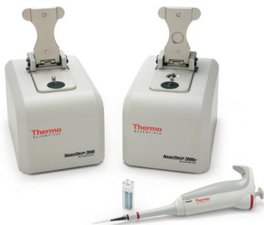
Using the patented NanoDrop microvolume sampling technology, a 1  $\mu\text{L}$  sample can be measured in less than 5 seconds. Simply pipette a 1  $\mu\text{L}$  sample directly onto the pedestal, measure and wipe clean. In addition to the pedestal, the NanoDrop 2000c instrument offers a cuvette position for larger volumes.
