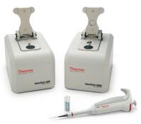
Using the patented Thermo Scientific NanoDrop<sup>™</sup> microvolume sampling technology, a 1  $\mu$ L sample can be measured in less than 5 seconds. Simply pipette a 1  $\mu$ L sample directly onto the pedestal, measure, and wipe clean. In addition to the pedestal, the NanoDrop 2000c instrument offers a cuvette position for larger volumes.
